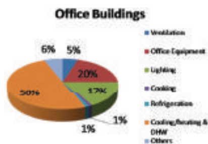
Energy consumers of an office building
